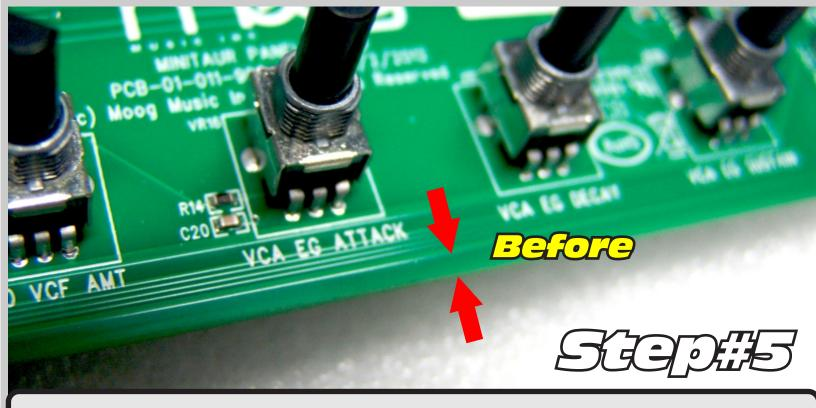
First we will focus on the bottom, the circuit board. The first thing we can do is sand down a couple of millimeters. The pic above shows the un-altered board. The bottom pic is after sanding. You can sand down VERY close and still not touch the bottom trace.
