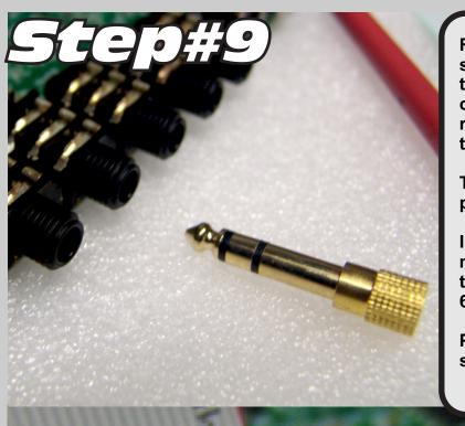
First we need to add the 'shorting' vinyl stickers. When no plug is inserted into the jack the metal fingers reach over and make connection to the other side. We will be removing these 'shorts' and then reattach them to our new jacks.
