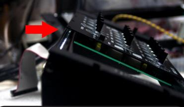
Test your final rack opening by taking a couple of washers and nuts and attach the front panel. This is temporary.
